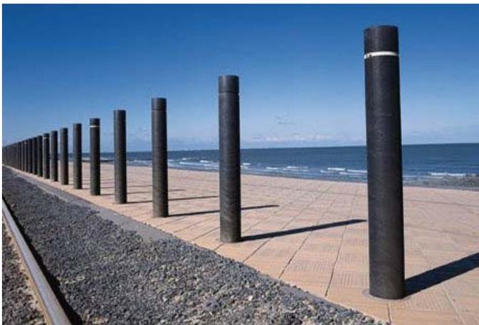
**Ornamental Recycled Plastic Bollards:** Constructed from solid recycled plastic, these bollards are durable and very strong. They are impervious to weather and salt laden air, and won't rust, fade or corrode. No painting, preservatives or maintenance is needed, and they can be colour coded with reflective rings. The bollards have a high strength galvanised steel core, and can be concreted on site to provide a ram-raid deterrent.
